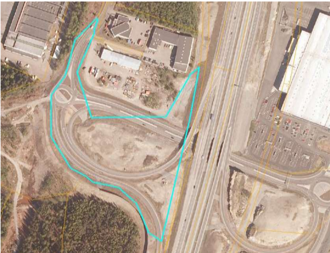
Wrong delineation, road network inaccurate and incorrect class code.
